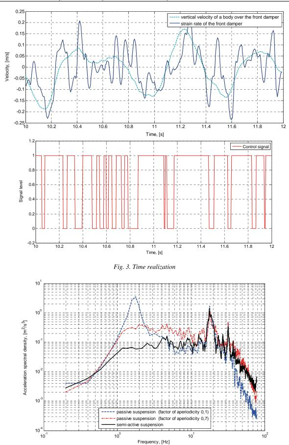
Fig. 4. Spectrums of vertical accelerations on a place of the driver
