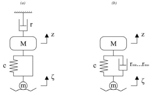
Fig. 1. Ideal sky-hook damping 1(a) and practical implementation of sky-hook damping 1(b)
